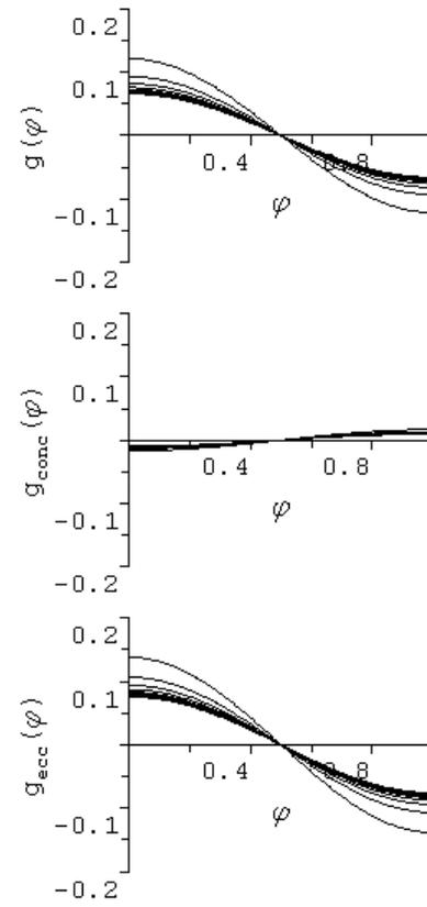
**Figure 11.** Parametric variations in  $g(\phi)$ ,  $g_{conc}(\phi)$  &  $g_{ecc}(\phi)$  with displaced fluid inverse power law index  $m_2$ :  $m_2 = 1.0, 1.3, 1.6, \dots, 4.0$ ;  $g_{conc}(\phi)$  flattens,  $g_{ecc}(\phi)$  flattens. Fixed parameters:  $\beta = 0.1$ ,  $e = 0.05$ ,  $b = -1$ ,  $\tau_{1,Y} = 1$ ,  $\kappa_1 = 1$ ,  $m_1 = 1$ ,  $\tau_{2,Y} = 0.8$ ,  $\kappa_2 = 0.8$ .
