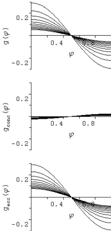
**Figure 8. Parametric variations in  $g(\phi)$ ,  $g_{conc}(\phi)$  &  $g_{ecc}(\phi)$  with buoyancy:  $b = 0.0, -0.25, -0.5, \dots, -2.5$ ;  $g_{conc}(\phi)$  elongates negatively,  $g_{ecc}(\phi)$  flattens. Fixed parameters:  $\beta = 0.1$ ,  $e = 0.05$ ,  $\tau_{1,Y} = 1$ ,  $\kappa_1 = 1$ ,  $m_1 = 1$ ,  $\tau_{2,Y} = 0.8$ ,  $\kappa_2 = 0.8$ ,  $m_2 = 1.0$ .**
