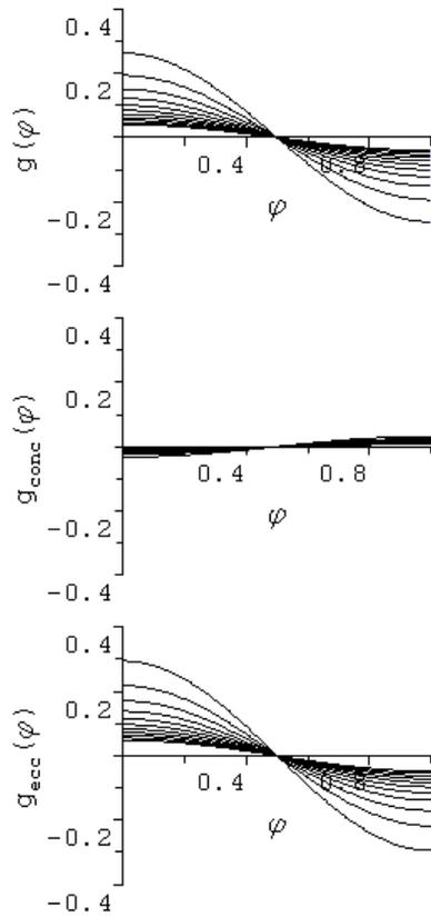
**Figure 10.** Parametric variations in  $g(\phi)$ ,  $g_{conc}(\phi)$  &  $g_{ecc}(\phi)$  with displaced fluid consistency  $\kappa_2$ :  $\kappa_2 = 0.1, 0.2, 0.3, \dots, 1.1$ ;  $g_{conc}(\phi)$  elongates negatively,  $g_{ecc}(\phi)$  elongates positively. Fixed parameters:  $\beta = 0.1$ ,  $e = 0.05$ ,  $b = -1$ ,  $\tau_{1,Y} = 1$ ,  $\kappa_1 = 1$ ,  $m_1 = 1$ ,  $\tau_{2,Y} = 0.8$ ,  $m_2 = 1.0$ .
