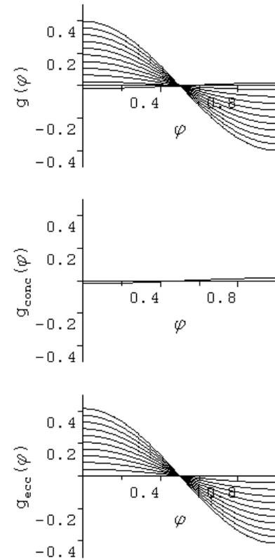
**Figure 7.** Parametric variations in  $g(\phi)$ ,  $g_{conc}(\phi)$  &  $g_{ecc}(\phi)$  with eccentricity,  $e$ :  $e = 0.0, 0.015, 0.03, \dots, 0.15$ ;  $g_{conc}(\phi)$  is unaffected,  $g_{ecc}(\phi)$  elongates positively. Fixed parameters are:  $\beta = 0.1$ ,  $b = -1$ ,  $\tau_{1,Y} = 1$ ,  $\kappa_1 = 1$ ,  $m_1 = 1$ ,  $\tau_{2,Y} = 0.8$ ,  $\kappa_2 = 0.8$ ,  $m_2 = 1.0$ .
