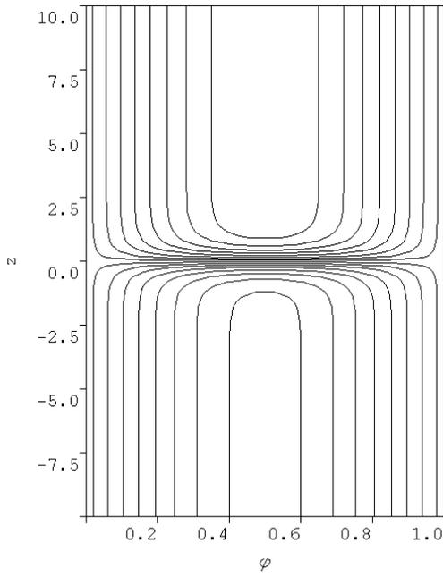
**Figure 5.** The function  $\Phi$ , for parameters:  $e = 0.1$ ,  $L = 10$ ,  $\tau_{1,Y} = \kappa_1 = m_1 = 1$ ,  $\tau_{2,Y} = 0.9$ ,  $\kappa_2 = 0.9$ ,  $m_2 = 1.1$ . Streamlines are spaced at intervals  $\Delta\Phi = 0.01$ .
