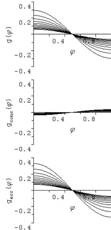
**Figure 9. Parametric variations in  $g(\phi)$ ,  $g_{conc}(\phi)$  &  $g_{ecc}(\phi)$  with displaced fluid yield stress  $\tau_{2,Y}$ :  $\tau_{2,Y} = 0.0, 0.15, 0.3, \dots, 1.5$ ;  $g_{conc}(\phi)$  elongates negatively,  $g_{ecc}(\phi)$  elongates positively. Fixed parameters:  $\beta = 0.1$ ,  $e = 0.05$ ,  $b = -1$ ,  $\tau_{1,Y} = 1$ ,  $\kappa_1 = 1$ ,  $m_1 = 1$ ,  $\kappa_2 = 0.8$ ,  $m_2 = 1.0$ .**
